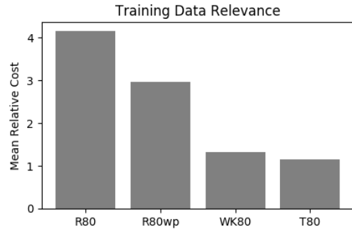
Figure 7: Relevance of training data vs. DQ’s plan cost. R80 is a dataset sampled independently of the JOB queries with random joins/predicates from the schema. R80wp has random joins as before but contains the workload’s predicates. WK80 includes 80 actual queries sampled from the workload. T80 describes a scheme where each of the 33 query templates is covered at least once in sampling. These schemes are increasingly “relevant”. Costs are relative w.r.t. EX.
